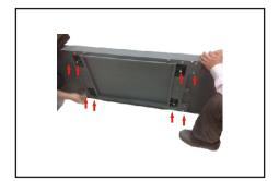
1. Place 16 M7x7. 5cm bolts 2. Bolts must be fully in position shown in image no. 1
