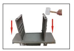
9. Install side walls as shown using a mallet and hit the side wall until firmly placed in position as shown
